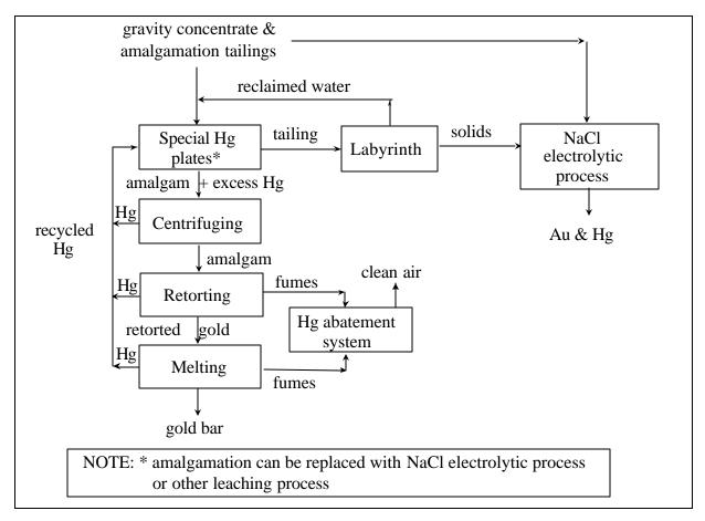
Fig. 6 - Steps in a UNECA Processing Center
