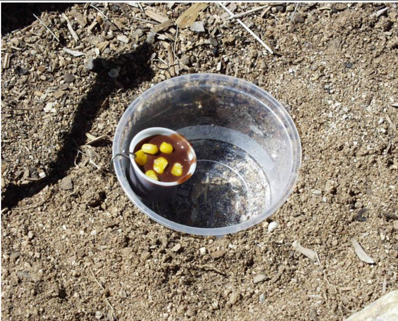
Once the Reifschneider Rain Shield is removed, the wire loop allows the dung cup to be swung out of the way, for easy - and clean - retrieval of specimens.
