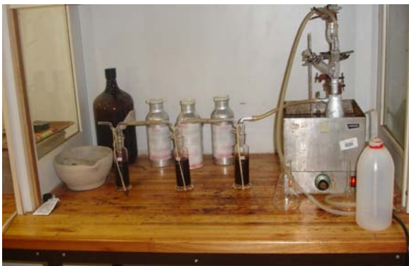
Phosphine gas reacting with Potassium permanganate (KMnO 4 ) solution
