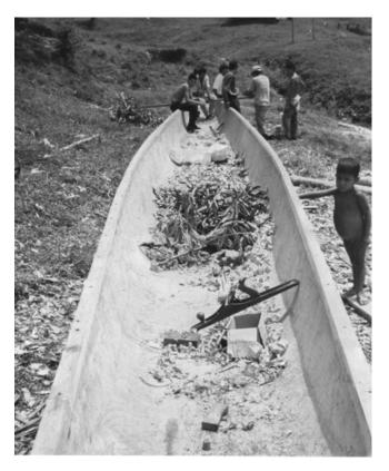
**Figure 1.** Tawahka men refining a freight river dugout at Krausirpi, Río Patuca, Honduras, 1996. The canoe is made from tropical cedar (*Cedrela odorata*), and is 44 feet (13.4 m) long with a beam of almost 4 feet (1.2 m).
