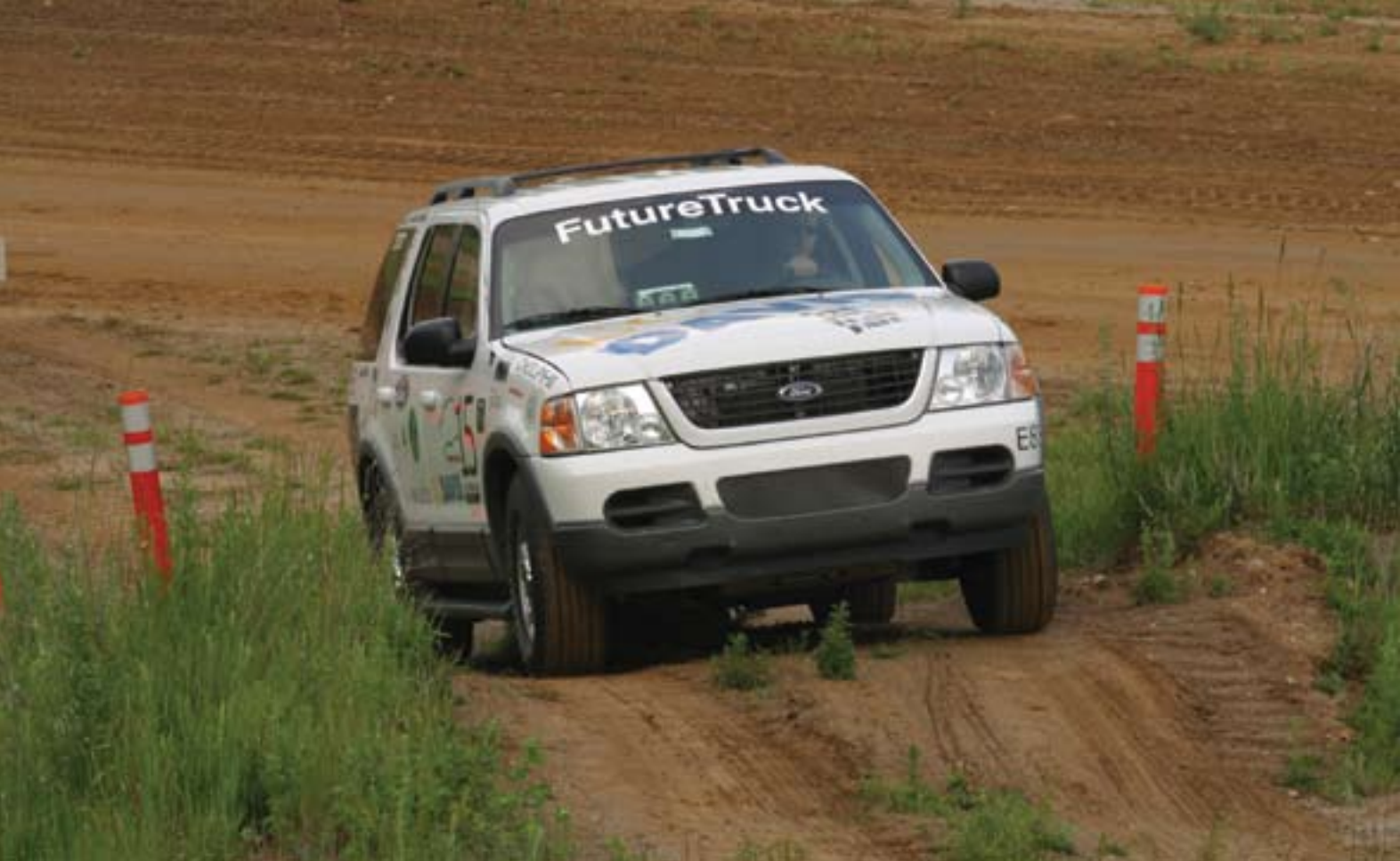
Figure 1. “Yosemite,” a Ford Explorer that was transformed into a plug-in hybrid, was tested at Ford’s proving grounds in Yucca, Arizona. This and similar prototypes have demonstrated the technology needed for a vehicle that can travel for several tens of miles on electric power alone while still having a small internal combustion engine available for longer trips. (Photograph courtesy of Argonne National Laboratory.)
