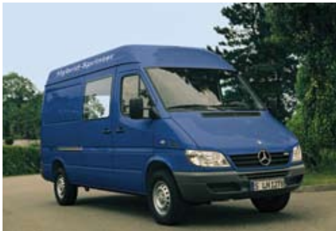
Figure 2. Only two plug-in hybrids are now commercially available: a special version of the Mercedes Sprinter delivery van (left) and an electric version of the Renault Kangoo (right) that carries a small internal combustion engine to charge its batteries, thus extending the car's range. (Photographs courtesy of DaimlerChrysler, left, and Renault, right.)
