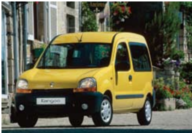
Figure 2. Only two plug-in hybrids are now commercially available: a special version of the Mercedes Sprinter delivery van (left) and an electric version of the Renault Kangoo (right) that carries a small internal combustion engine to charge its batteries, thus extending the car's range. (Photographs courtesy of DaimlerChrysler, left, and Renault, right.)
