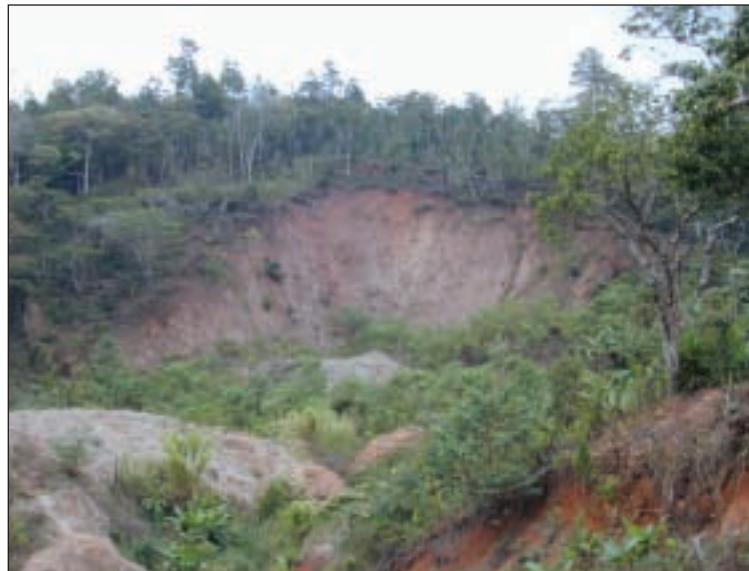
Figure 9. Headscarp (approximately 8 m high) of landslide in deeply weathered materials in northern Matagalpa study area.
