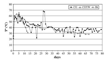
Fig. 2. Temperature evolution in composting experiments.
