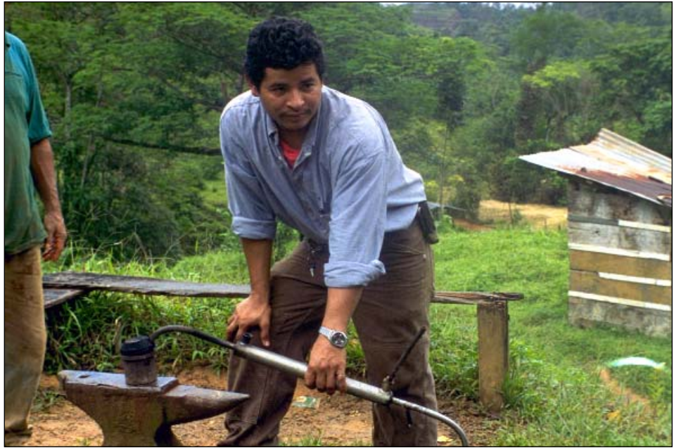
Illustrating the retort used to capture mercury vapour and to carry it into cold water where it again becomes liquid and can be recovered and reused.
