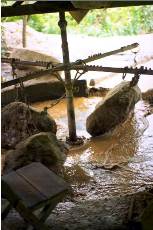
Grind rocks of a "rastra", grinding ore fine and mixing it with mercury. Rocks are lifted when the process is completed and the amalgam of mercury and gold is scraped from the rock floor.
