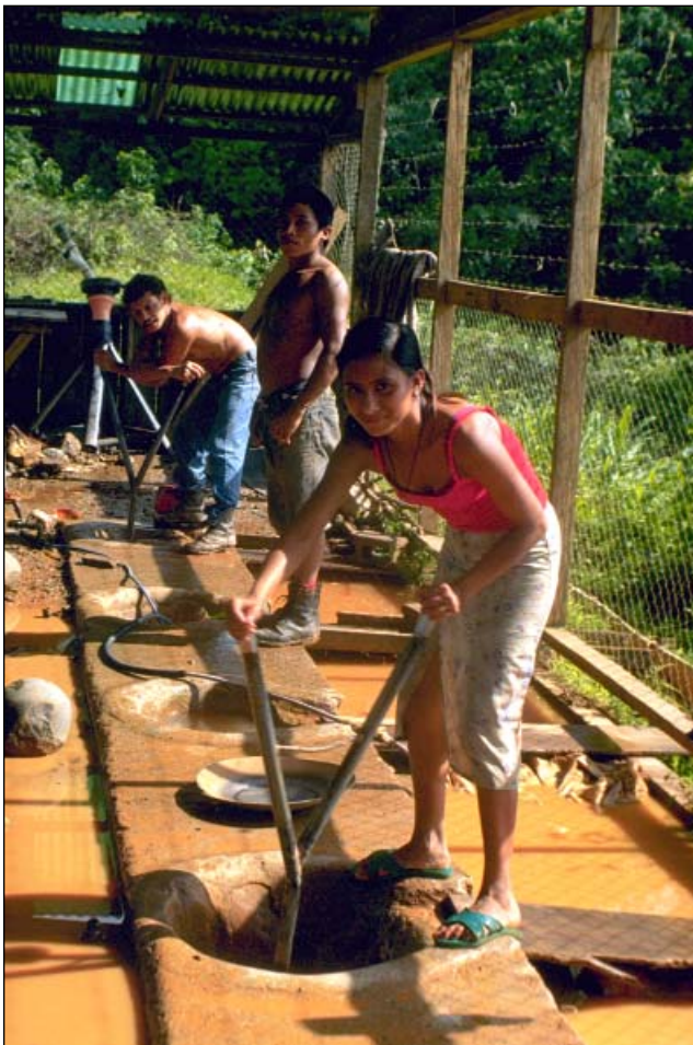
Manual ore-processing using "molinetes" for high-grade ore.
