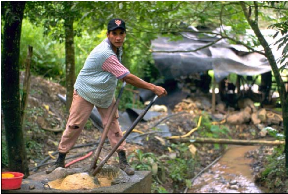
Processing high-grade ore using a "bolillo". Mercury is added to the finely ground ore.
