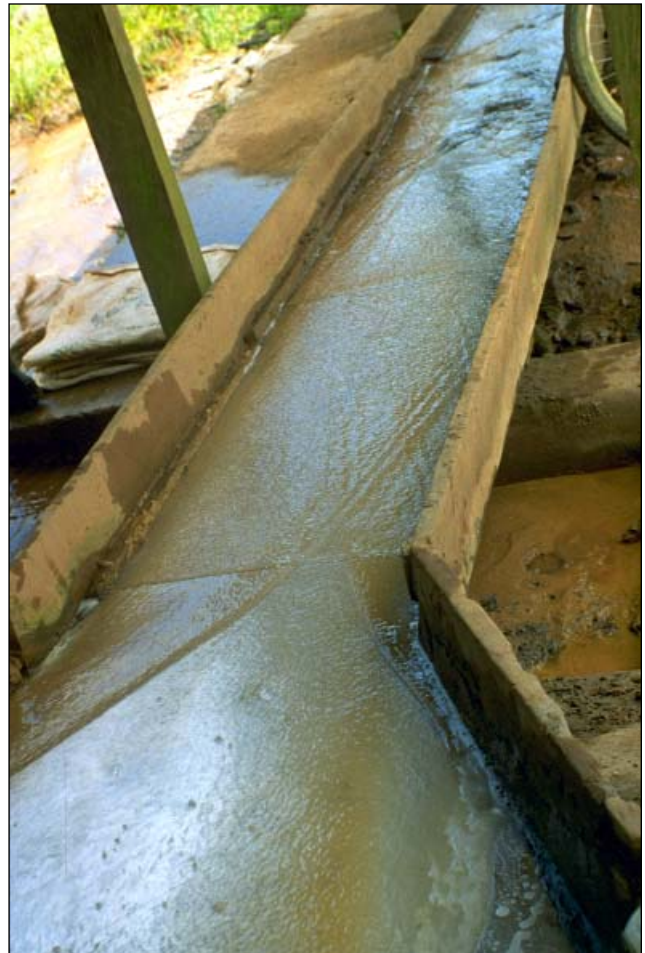
Trough coated with mercury, connected to the hammer mill at the DPM processing plant, Bonanza.
