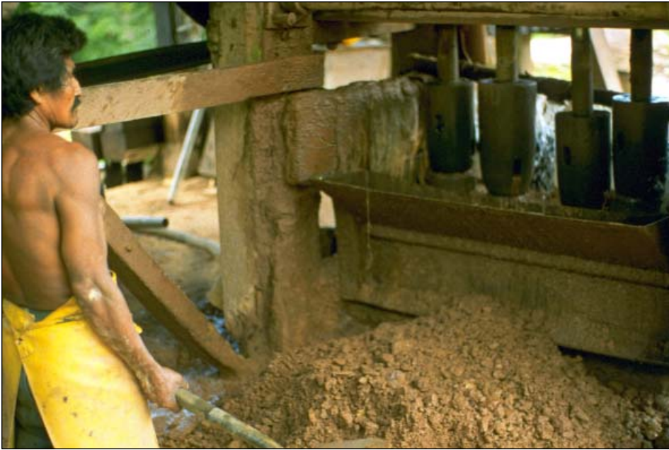
DPM ore-processing plant. Gold-rich ore is shovelled into this hammering mill for crushing and mixing with mercury.
