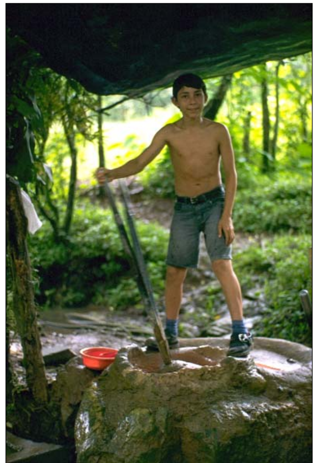
Processing high-grade ore using a "bolillo". Mercury is used to draw out the gold from the finely ground ore.
