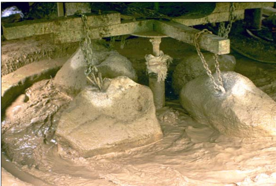
A traditional ore-processing "rastra", grinding high-grade ore.
