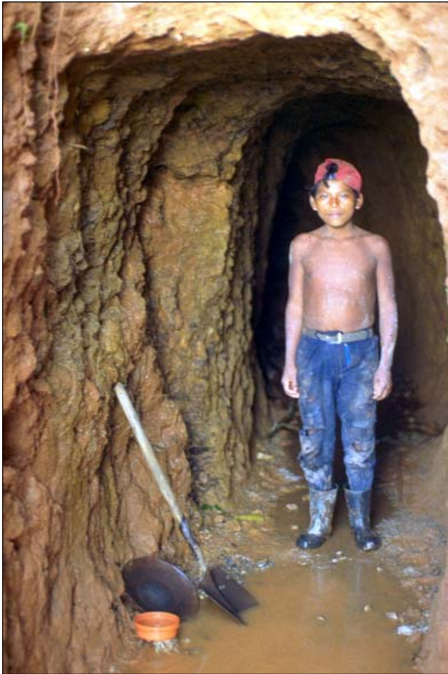
13 year-old boy extracting ore from this horizontal shaft. Notice that there is no wood reinforcing of tunnel walls.
