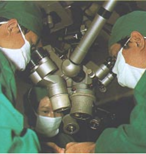
Fig. 4.18 Operating microscope — now used by most ophthalmic surgeons for all anterior segment operations.
