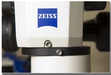
Photo 5: The intermediate mount shifts the mage path to align with the focusing path.
