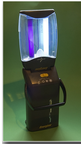
The lantern with the tubes inverted, allowing them to attract scarabs from both sides.
