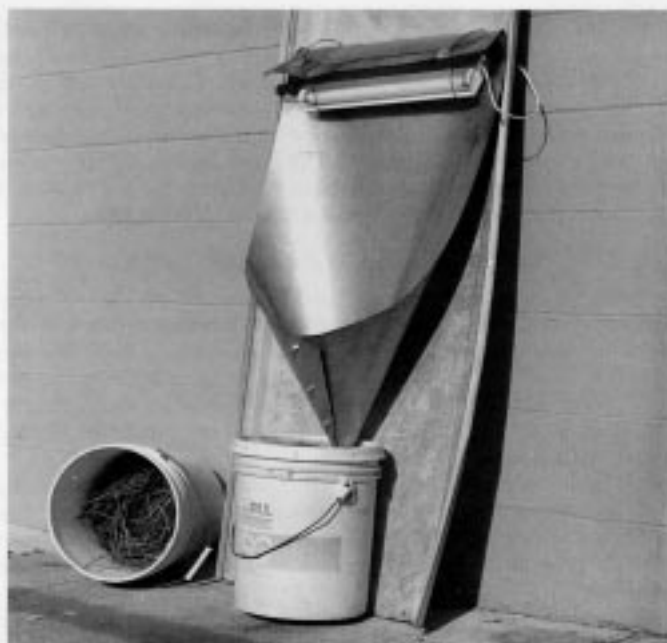
Fig. 7. Blacklight set-up showing tin funnel and extra bucket three-fourths filled with straw.
