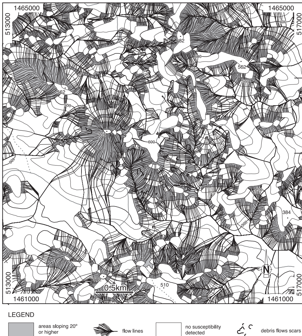
Fig. 6. Example of the susceptibility map corresponding to the Cinco Pinos area (locality in Fig. 4A). Areas highlighted in grey correspond to the ones sloping equal to or higher than 20^\circ , and are the ones considered susceptible to failure. Flow lines correspond to possible debris flow paths, taking the areas highlighted in grey and mapped scars as possible source areas. See text for detailed discussion.
