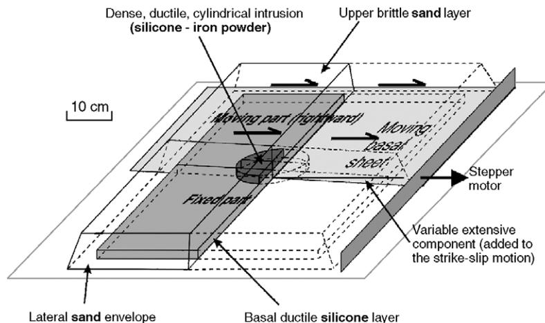
Fig. 4. Experimental setup.
