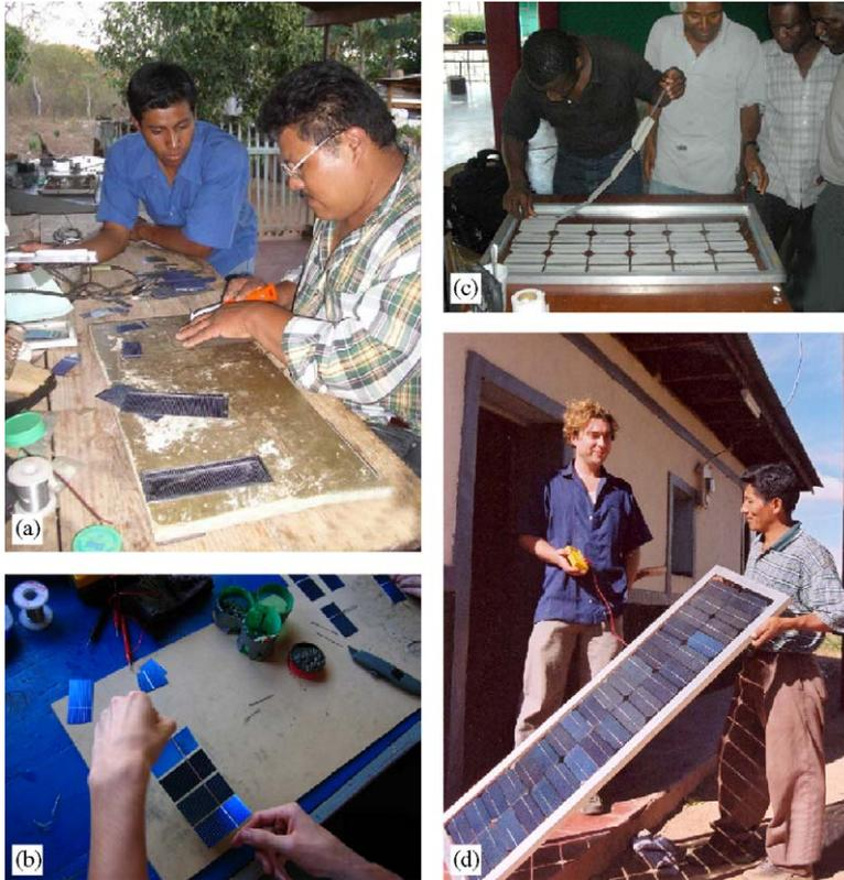
Fig. 1. Module encapsulation process description. (a) Cutting the cells, (b) soldering, tabbing and stringing the cells, (c) casting the strings into a silicone bath and (d) testing the panel in natural sunlight.
