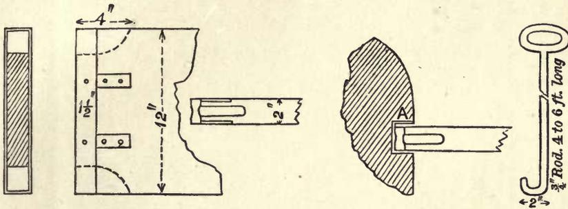
it here more as a bit of information as to what can be done, than to detract from the invention alongside. This is useful in cases of very deep water where a rod would be long and unwieldy, but the fact that the catch on the plank is *in* the groove in the pier makes it easy to find.
