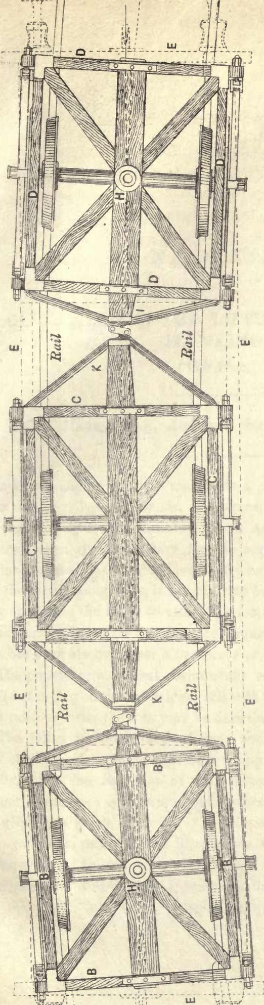
PLAN OF AXLE FRAMES ON A CURVE OF 100 FEET RADIUS
