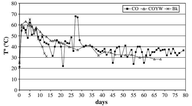
Fig. 2. Temperature evolution in composting experiments.
